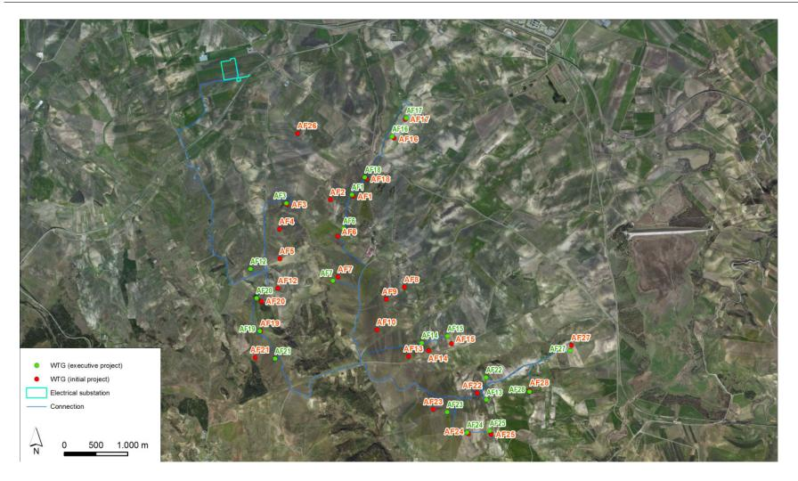
After the first application for the installation of 27 WTGs of 3,3 MW each one for a total power of 89,1 MW (red WTGs in the figure above), the project is changed in terms of layout and power (the final layout is composed of 20 WTGs of 3,00 MW each for a **total power of 60 MW (**green WTGs in the figure).
