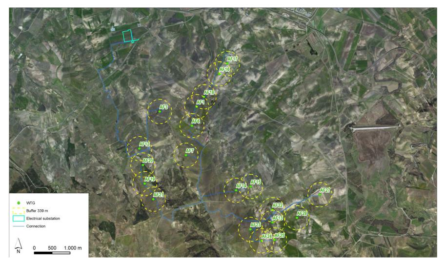
For the windfarm >1 MW, the Regional Energetic Plan (named PIEAR) requires that the WTG distance has to be > 3 Diameter of the Rotor (113 meters x = 339 m). The windfarm is in compliance with the PIEAR.
